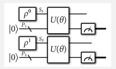
The quantum circuit to estimate trace distance. The two qubits are measured and the verifier accepts if the measurement outcome is 0 on first qubit and 1 on second qubit.
